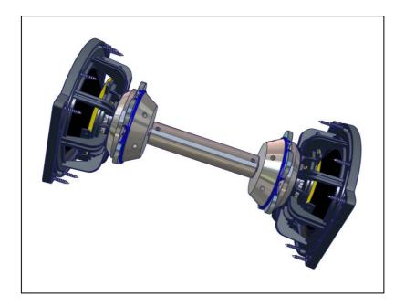
The design of this subwoofer incorporates dual drive units, operating in tandem, which fire the sound on two planes. The mechanical connection of the two drive units (enabled by means of a rigid connection component) avoids unwanted cabinet resonances.
